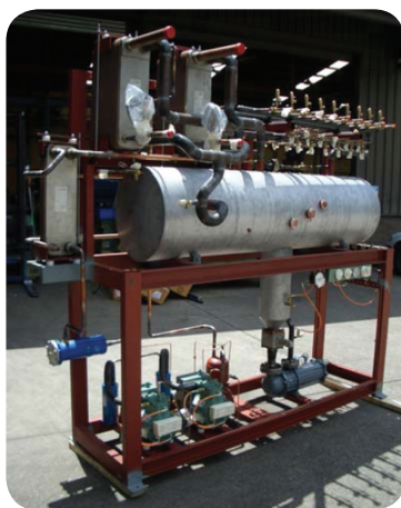
Picture 14 – Detail of rack with pumping system of liquid CO 2
