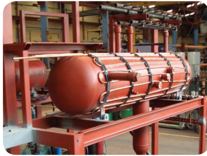
Picture 12 – An example of a serpentine coil application used to keep CO 2 cold in case of electrical failure. It should be connect to a condenser unity driven by generator
