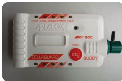
Picture 16 – Example of a detector of CO 2 leakage
